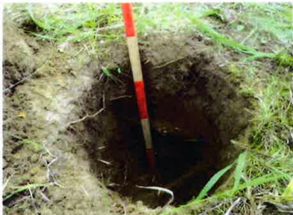
Plate 3: Test pit in a disturbed area, Block 11, facing southeast. Note that matrix is homogenous fine sand.
