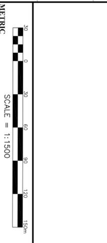
DISTANCES SHOWN ON THIS PLAN ARE IN METRES AND CAN BE CONVERTED TO FEET BY DIVIDING BY 0.3048
