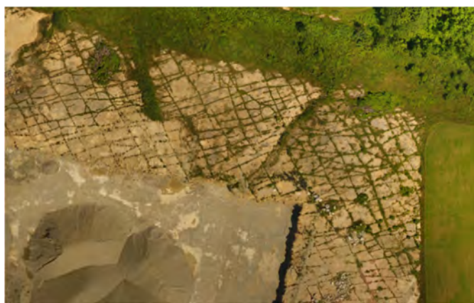
FIGURE 4: BEDROCK ROCK SURFACE AND VERTICAL JOINTING
