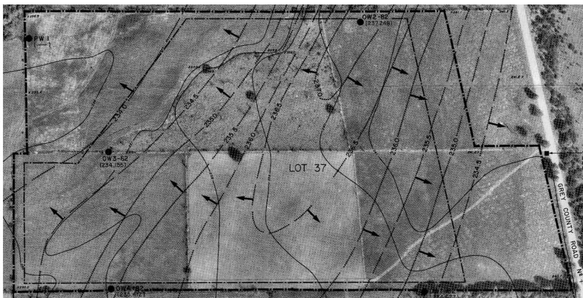
FIGURE 10: GROUNDWATER FLOW MAP (PRE-SARAWAK QUARRY)
