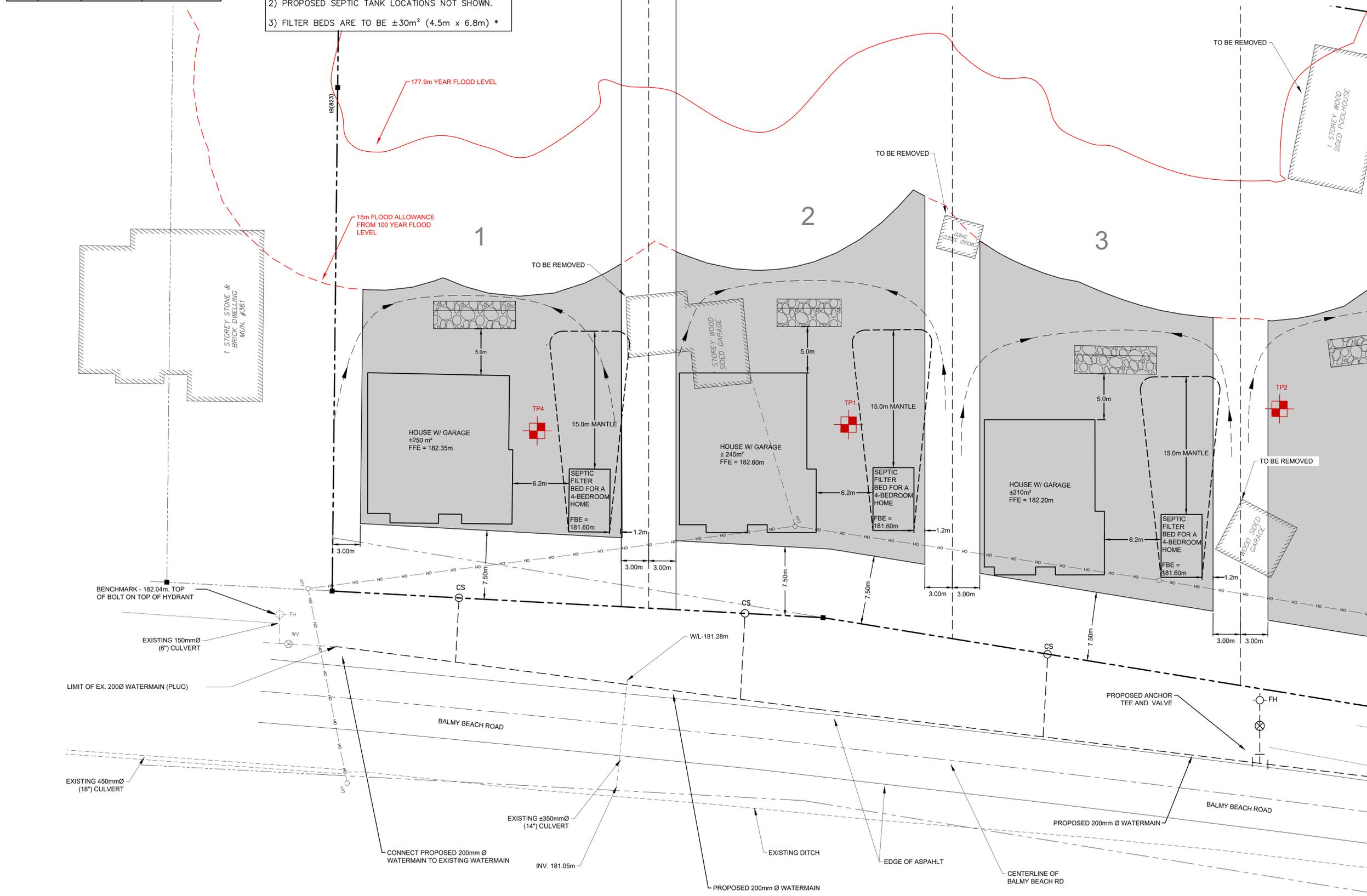
\* FILTER BED BASED ON A 4 BEDROOM HOME WITH A DAILY FLOW OF 2000 L/DAY. USE A = Q/75 = 2000/75 = 26.72 m<sup>2</sup> (MINIMUM OF 30 m<sup>2</sup> RECOMMENDED).
